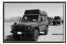
One of those advantages is the armour protection systems kit. Tailor designed so complete sections of the vehicle—such as doors and windshield—can be removed and replaced by armoured modules, it will provide NATO level 1 protection against small arms and protection against hand grenades and anti-personnel mines. Additional armoured components are included to protect the floor, roof and rear wall of the crew area.
